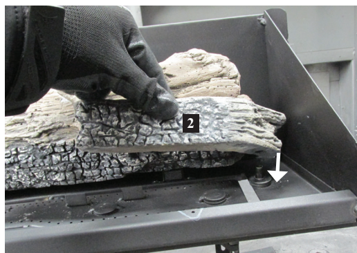
Logs 2 - fits over pin on left side - rests against tab on right
